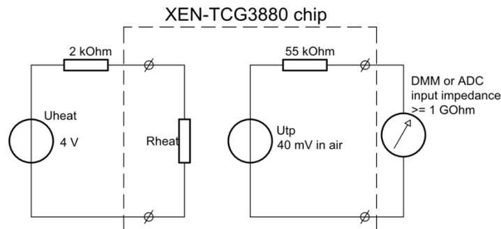
**Figure 1:** Constant voltage biasing of the XEN-3880 with 2 kOhm series resistance for minimizing temperature effects on the output voltage in case of gas type measurement.
