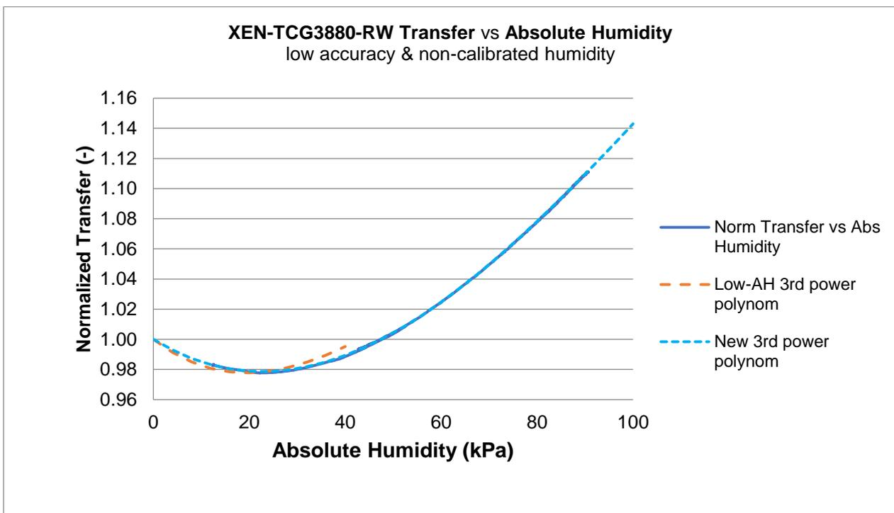
Figure 1: Typical XEN-TCG3880 normalized transfer as a function of partial pressure of water vapor (red curve measured at up to 80 °C, blue curve measured at 100 °C). The right part of the blue curve, striped, shows the extrapolated curve based on a 3<sup>rd</sup> power polynomial.
