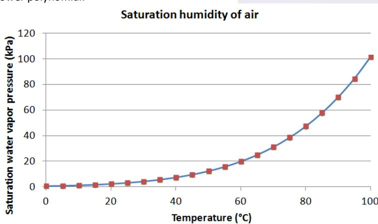
Figure 2: Saturation partial pressure of water vapor vs temperature.
