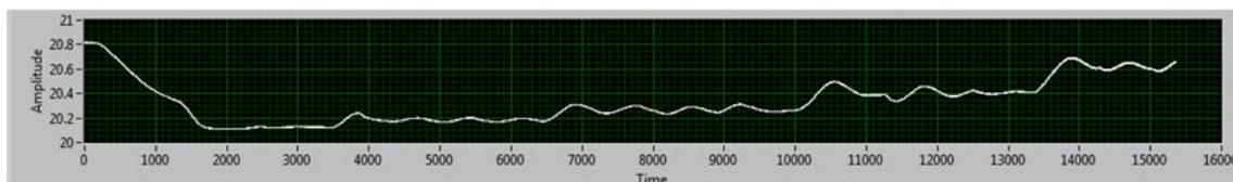
**Figure 3:** Transfer of the XEN-3880 for measurements at ever increasing absolute humidity in kPa. Transients in humidity do not show in the transfer of the XEN-5320 around 20 kPa partial water vapor pressure (measurement 2000-3000), but do show when the humidity levels are higher (later measurements), as indicated in Fig. 1. Also the absolute value of the transfer increases at higher measurement (= water vapor partial pressures) numbers, as indicated in Fig. 1.
